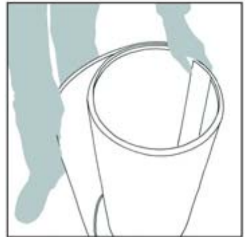
Roll up graphic panels one by one. Graphics on outside, magnetic strips on inside.
